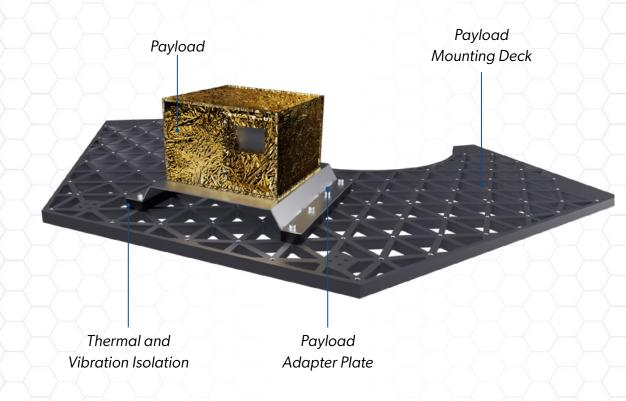
Additionally, the adapter plate can be utilized to dampen loads as experienced by the payload. It can also simplify the provision of the required thermal characteristics as well as the implementation of the required grounding, bonding, and isolation techniques at the payload mounting interface to the lander.
