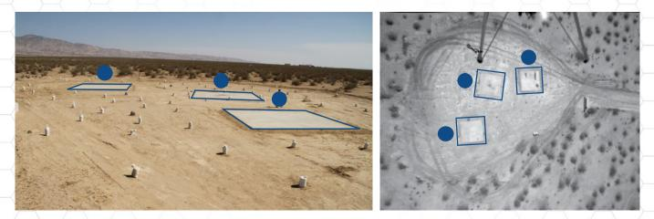
Early version of the OPAL sensor autonomously selects a hazard-free landing site for the Masten Space Systems Xombie Rocket.
