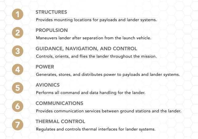
The following pages highlight the polar configuration of the Griffin bus as utilized on Griffin Mission One to deliver the NASA VIPER rover to the lunar South Pole. Additional configurations for lunar orbit, equatorial, far side, and many more delivery locations are possible. Contact Astrobotic for more details on specific configurations.
