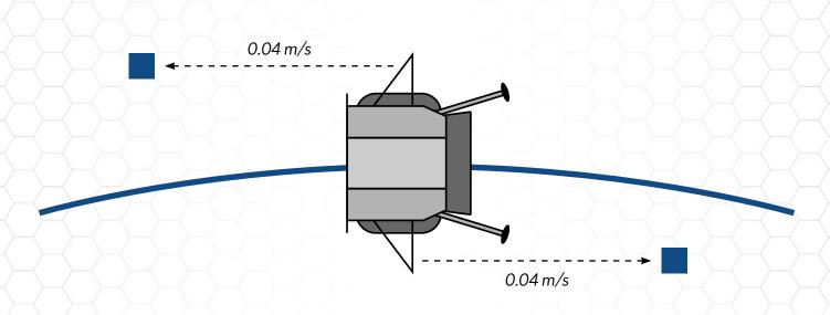
The lander nominally holds in several different lunar orbits during the Lunar Orbit phase; not all lunar orbits are available for orbital payload deployment as some may be less stable than others. Astrobotic identifies the available and preferred lunar orbits for payload customer orbital deployments for each mission. To ensure safe lunar orbit operations for all payloads, orbital deployments may occur at slightly varied altitudes for each payload.
